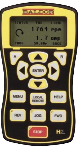
keys along with left and right arrows **navigate effortlessly** through the display and programming functions.
