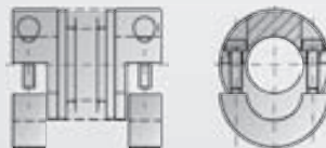
miniature bellows coupling with split hubs
